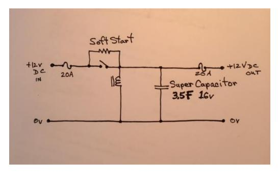
The Soft Start circuit is used to initially charge the capacitor. Inrush current can be in the 100A range if not limited.
