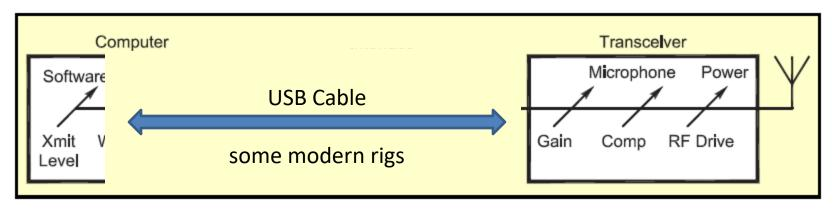
An example of daisy-chained transmit level controls. Note that the controls are in series and the resultant output is affected by each of the prior control settings.
