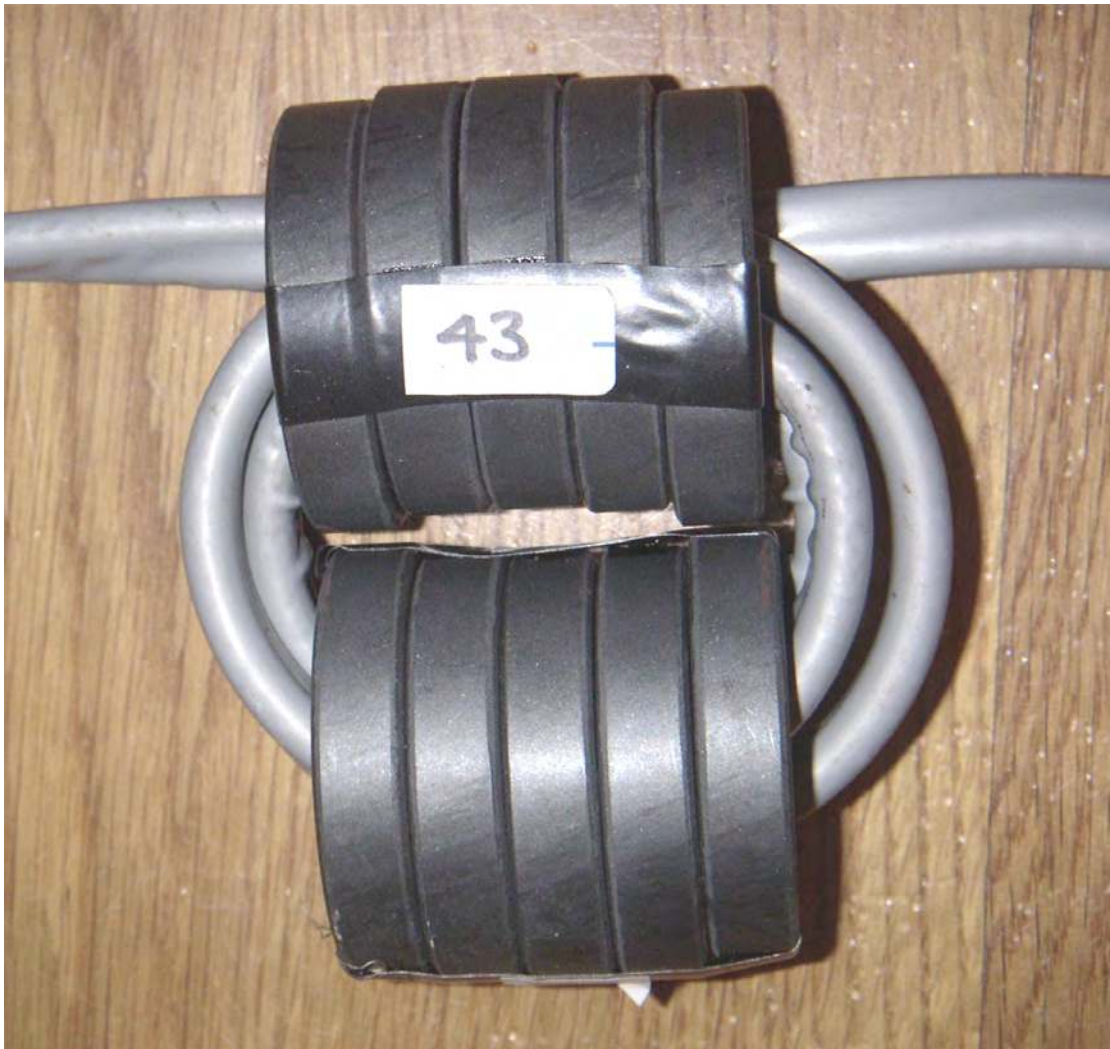
Figure 13: Common-mode choke for a 2 \times \text{AWG } 4 , DC power cable, formed by threading the cable 3\frac{1}{2} times through a binocular core formed by two stacks of five Fair-Rite p/n 5943003801, mix-43, “ring” toroids.
