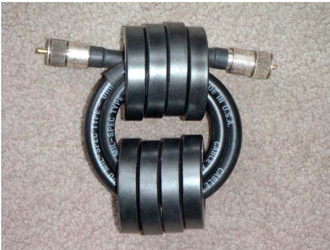
Figure 4: Common-mode choke for high HF power, formed by passing RG-213/U coaxial cable 3\frac{1}{2} times through a binocular core formed by two stacks of four Fair-Rite p/n 5943003801, mix-43, toroids. This choke's impedance exceeds 1\text{ k}\Omega from 1.8 through 18 MHz, dropping to 550\text{ }\Omega at 30 MHz. One such choke should be installed at the antenna feedpoint, one at the amplifier output, and at least one other in-between.
