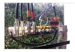
On the inside shown above, the rotor cable comes in through the hole that was for the "F-connector" and goes to a terminal block where there are 37volt MOVs and .01 caps on each of the 8 lines. Above the terminal block is a Molex connector used as the quick disconnect for the rotor cable.
